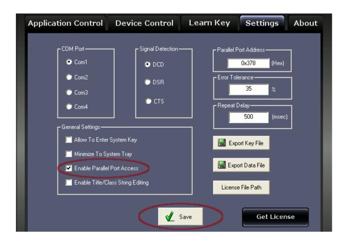
Once the access is enabled come back to "Device Control" tab. You may find that current data on the parallel port is reflected on the parallel-port-status (as shown
